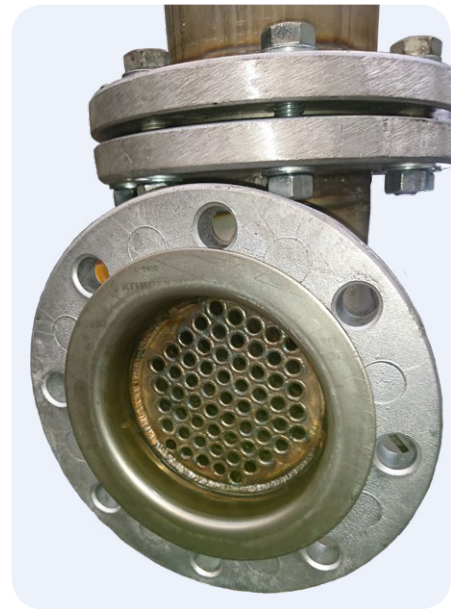
Heat exchanger (supply side)
